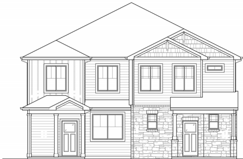
3 FRONT ELEVATION BUILDING TYPE C NTS
