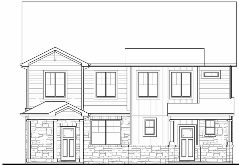
1 FRONT ELEVATION BUILDING TYPE A NTS
